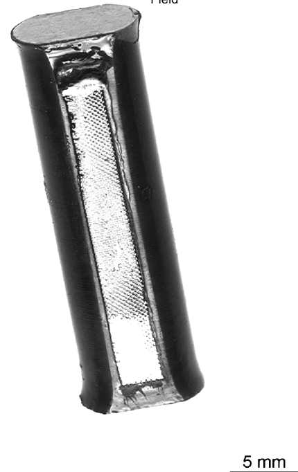
Fig. 11. (a) Bi-polar strain field behavior in a multilayer copper electrode actuator, and (b) multilayer copper electrode PZT actuator.
